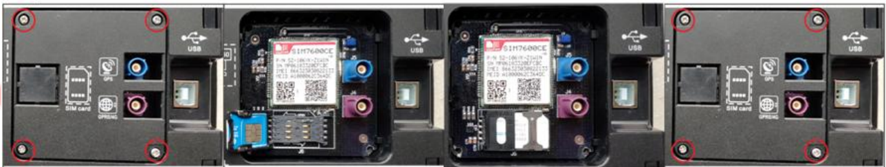
Fig. 14 SIM Card Installation Method
