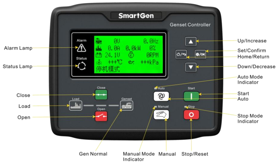
Fig.1 - HGM6110LT Front Panel Indication
