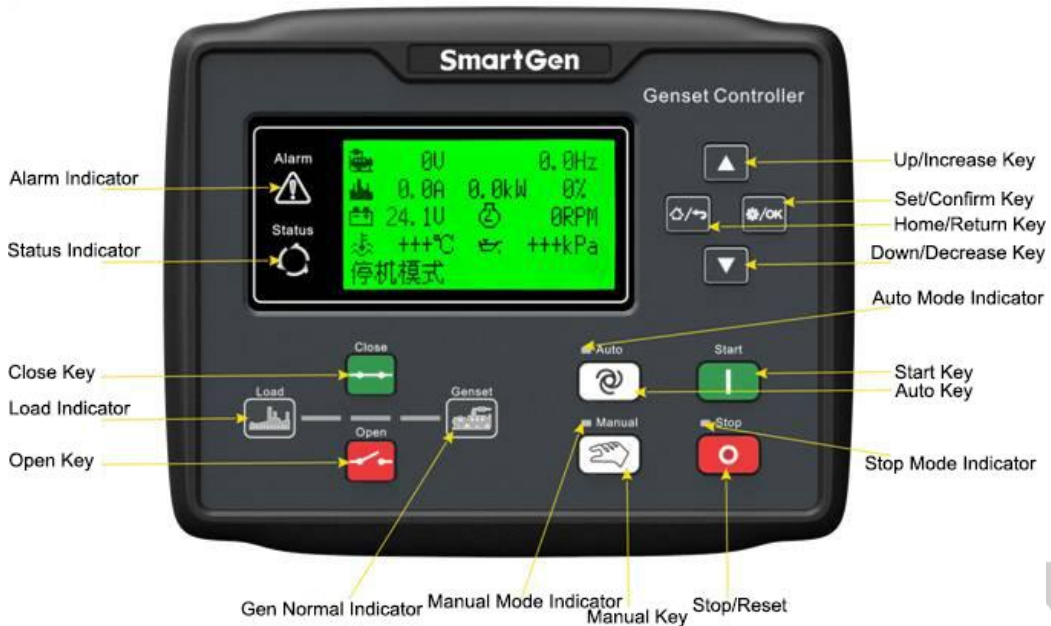
Fig. 1 HGM6110N-RM Front Panel Indicators
