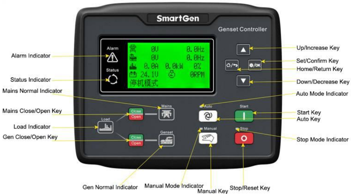
Fig. 2 HGM6120N-RM Front Panel Indicators
